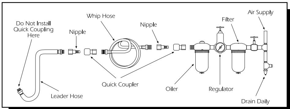
Tools of this class operate on a wide range of air pressures. It is recommended that air pressure of these tools measure 90 PSI at the tool while running free. Higher pressure (over 90 psig; 6.2 bar) raises performance beyond the rated capacity of the tool, which will shorten tool life because of faster wear and could cause injury.
