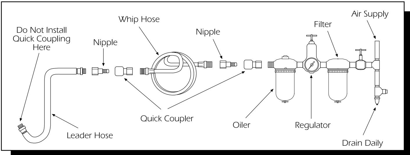
Tools operate on a wide range of air pressures. It is recommended that air pressure measures 90 psig at the tool with the trigger fully depressed and no load applied to the tool. Higher pressure (over 90 psig; 6.2 bar) raises performance beyond the rated capacity of the tool, which will shorten tool life and could cause injury.
