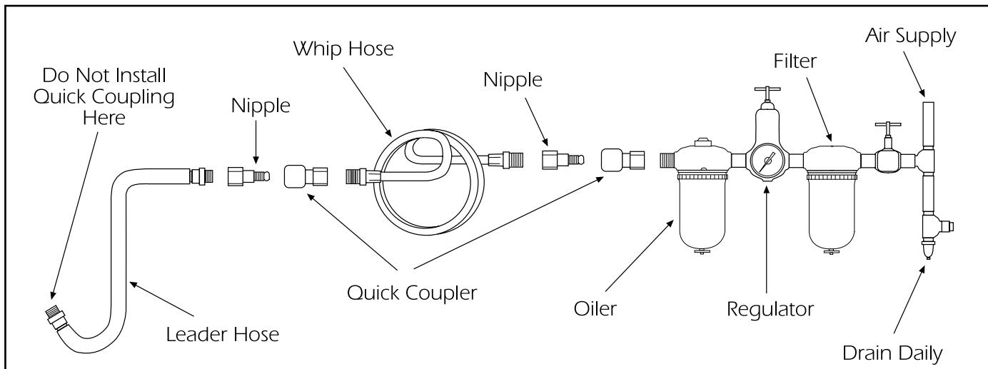
Tools operate on a wide range of air pressures. It is recommended that air pressure measures 90 PSI at the tool with the trigger fully depressed and no load applied to the tool. Low pressure (under 90 psig; 6.2 bar) reduces the speed of all air tools. Low air pressure not only wastes time, but also costs money. Higher pressure (over 90 psig; 6.2 bar) raises performance beyond the rated capacity of the tool, which will
