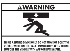
DO NOT OVERLOAD. OVERLOADING CAN CAUSE DAMAGE TO OR FAILURE OF THE JACK.
