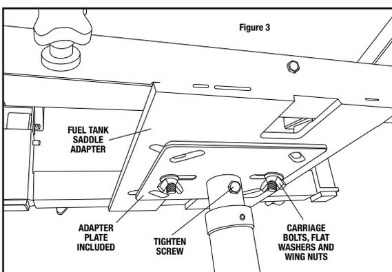
**TYPE 3** - Some jacks will have to have their stock saddles removed and replaced with the #10 adapter plate included with the saddle adapter. The adapter plate is secured to the jack's ram by tightening the #9 screw at the base of the adapter plate. See Figure 3. Follow the assembly instructions for TYPE 2 jacks to secure the saddle adapter to the adapter plate.
