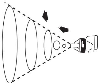
Spray pattern may be infinitely adjusted from round to flat.
