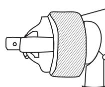
Set inlet pressure at no more than 43 PSI. For optimum performance, some materials may spray better at PSI ratings below 43 PSI. If unsure, always test at PSI ratings before using on final production. Try spray. If it is too fine, decrease the air pressure or open fluid control screw. If the spray is too thick, close the fluid control screw. Regulate the pattern width and repeat adjustment of spray as needed.
