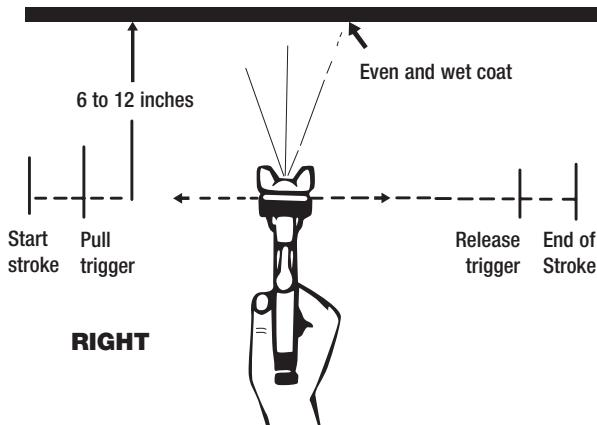
on material and atomizing pressure. For a uniform finish, lap each stroke over the preceding stroke, making sure the spray is smooth and wet.
