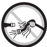
• Air under pressure can cause severe injury. Never direct air at yourself or others. Always turn off the air supply, drain hose of air pressure and detach tool from air supply before installing, removing or adjusting any accessory on this tool, or before performing any maintenance on this tool. Failure to do so could result in injury. Whip hoses can cause serious injury. Always check for damaged, frayed
