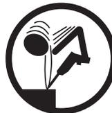
• Tool shaft may continue to rotate briefly after throttle is released. Avoid direct contact with accessories during and after use. Gloves will reduce the risk of cuts or burns.
